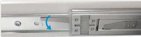
Release the locks on both sides by pulling down the levers on the rails and gently pushing the appliance until it reaches the rack front posts.
