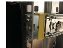
Once the rail guide is in place, slide again the yellow lock into locking position.
