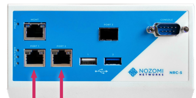
C. Plug the SFP modules into the slots if needed. Connect monitoring ports to the proper network mirror sources as needed.
